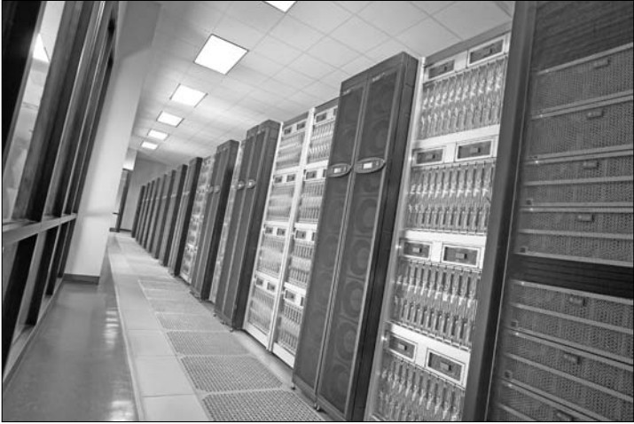
Figure 2-2: Ranger provides computational capabilities to the national research community and is built using the Sun Constellation System architecture from Sun Microsystems.
